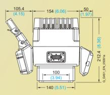
Inverter with PROFIBUS module (including PROFIBUS connector and T-piece - neither is included in the scope of supply) and EM module
