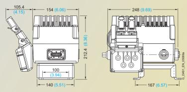
Inverter with PROFIBUS module (including PROFIBUS connector and T-piece - neither is included in the scope of supply)
