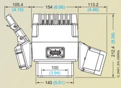
Inverter with PROFIBUS module (including PROFIBUS connector and T-piece - neither is included in the scope of supply) and REM module
