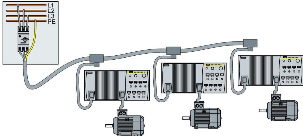
Image 3-9 Power supply to an inverter group via a shared 400-V branch circuit
