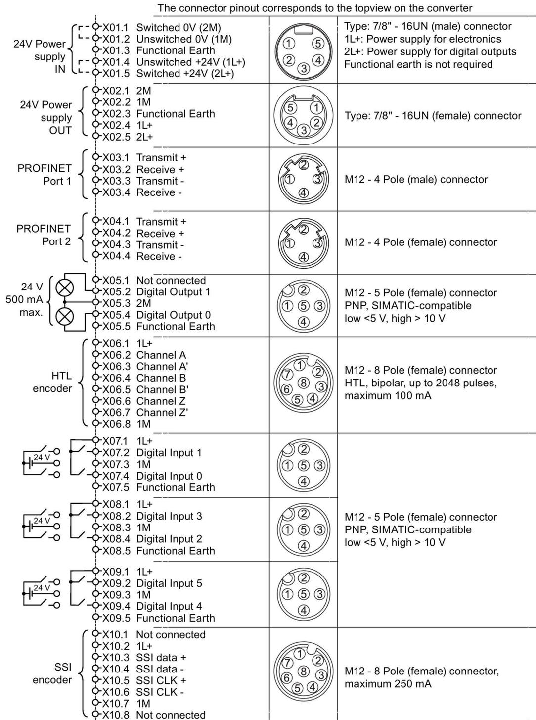
Image 3-15 CU250D-2 PROFINET connectors
