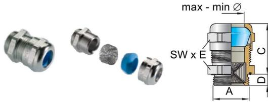
Image 3-6 Example of a Blueglobe EMC cable gland
