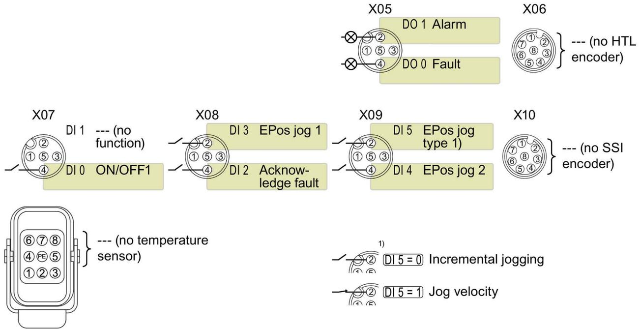
Image 3-20 Factory settings of the CU250D-2 control units
