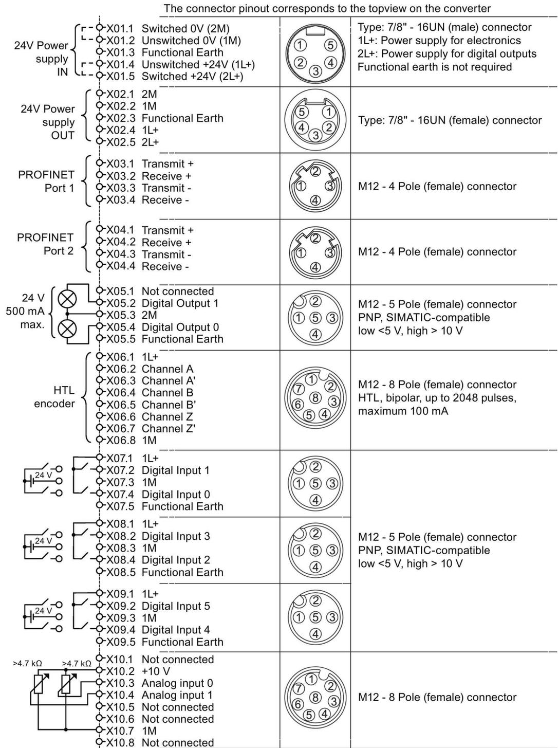
Image 3-11 CU240D-2 PROFINET connectors
