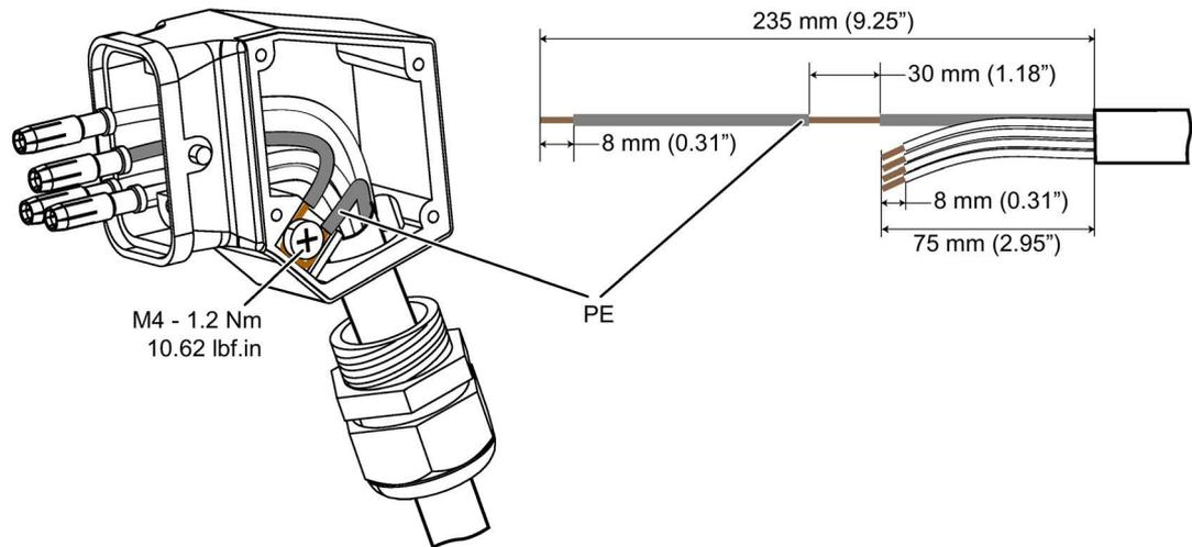
Image 3-5 Grounding the line supply and motor connectors
