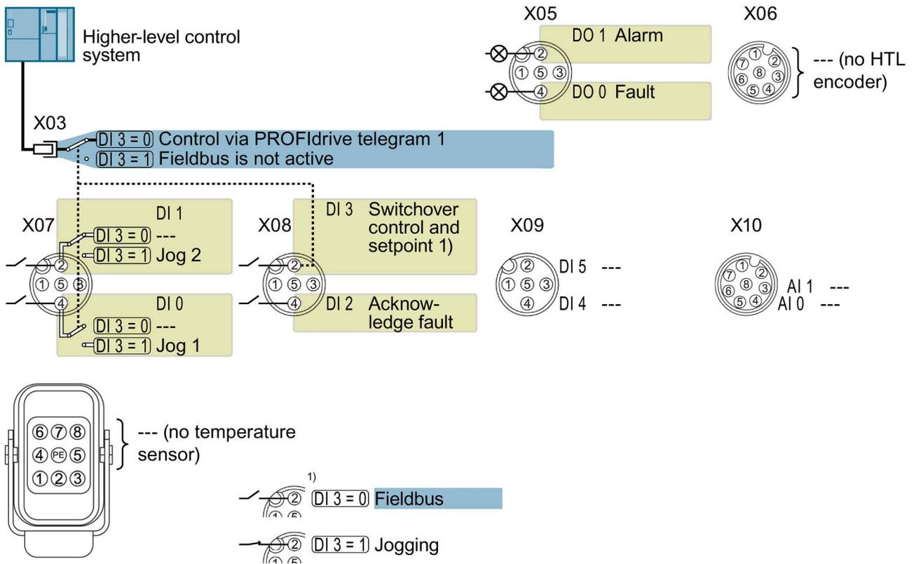
Image 3-19 Factory settings of the control units CU240D-2
