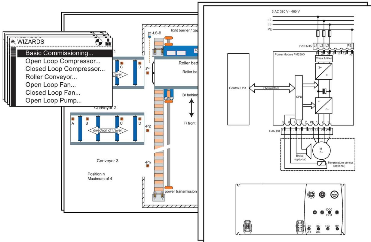
Image 4-2 Example of IOP Wizards and Inverter wiring diagrams
