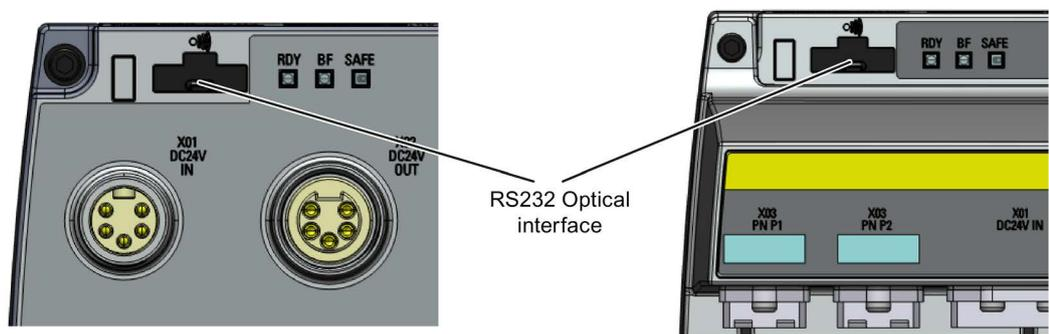
Image 4-1 CU240D-2 and CU250D-2 Optical Interfaces
