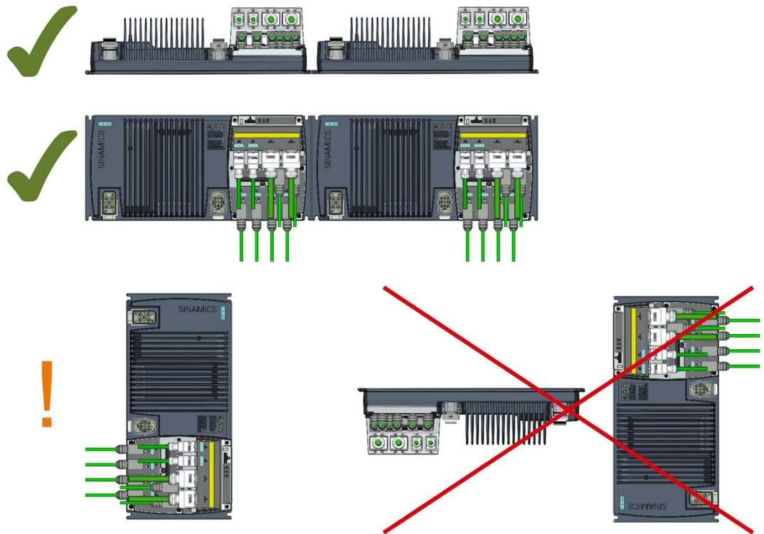
Image 3-3 Mounting orientation: correct (✓), impermissible (X), permissible with restrictions (!)
