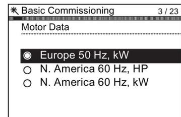
5. Select the correct frequency for your Inverter and attached motor.
