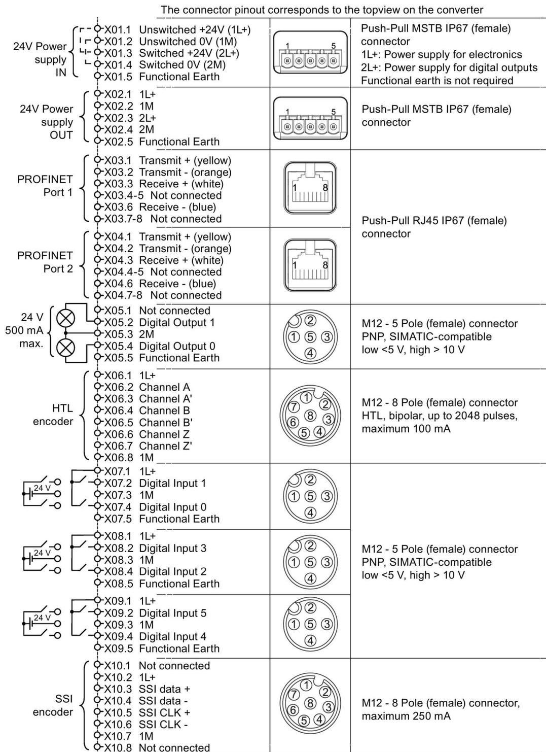
Image 3-16 CU250D-2 PROFINET Push-Pull connectors
