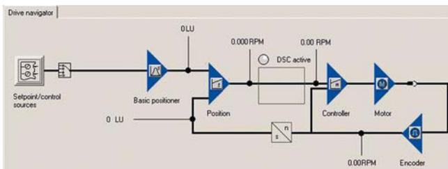
The EPos basic positioner in the SINAMICS drive system provides powerful and precise positioning functions. Due to its flexibility and adaptability, the basic positioner can be used for a wide range of positioning tasks.
