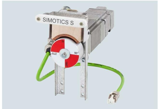
The servo module expands the single-axis drive modular training case with servo functionality. The servo module comprises a SIMOTICS S-1FK7 servomotor with load equipment and a mounted mechanical system. The encoder cable is integrated into the servo module. The power cable is already included in the scope of supply of the SINAMICS modular training case.
