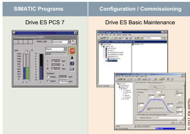
Drive ES is the engineering system used to integrate the communication, configuration and data management functions of Siemens drive technology into the SIMATIC automation world easily, efficiently and cost-effectively.
