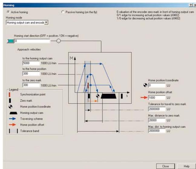
The EPos basic positioner in the SINAMICS drive system provides powerful and precise positioning functions. Due to its flexibility and adaptability, the basic positioner can be used for a wide range of positioning tasks.
