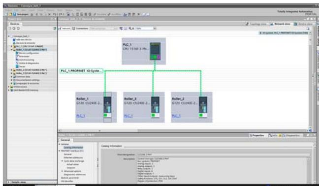
SINAMICS Startdrive is a tool for configuring, commissioning, and diagnosing the SINAMICS family of drives and is integrated into the TIA Portal.
