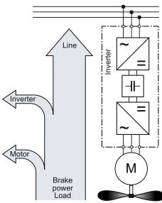
Braking with regenerative feedback into the line supply
