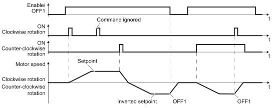
Figure 7-5 Three-wire control, method 1
