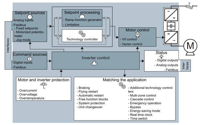
Figure 7-1 Overview of inverter functions
