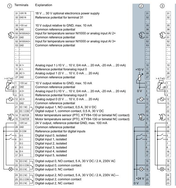
The wiring of the terminal strip is not shown completely, but as example for each terminal type.
