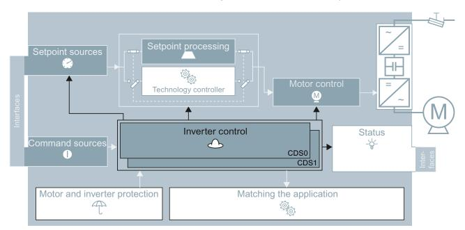
Figure 7-7 CDS switchover in the inverter
