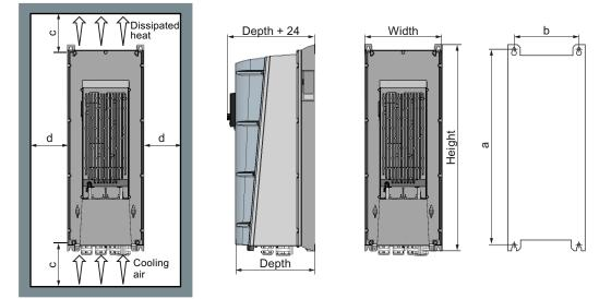
Figure 3-1 Drilling pattern for PM230
