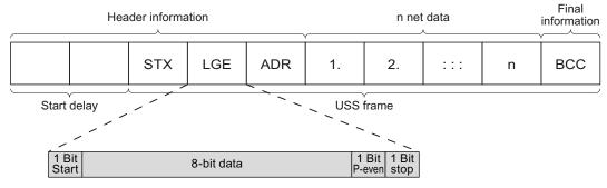
Figure 6-5 Structure of a USS telegram
