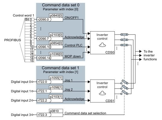
You select the command data set using parameter p0810. To do this, you must interconnect parameter p0810 with a control command of your choice, e.g. a digital input.
