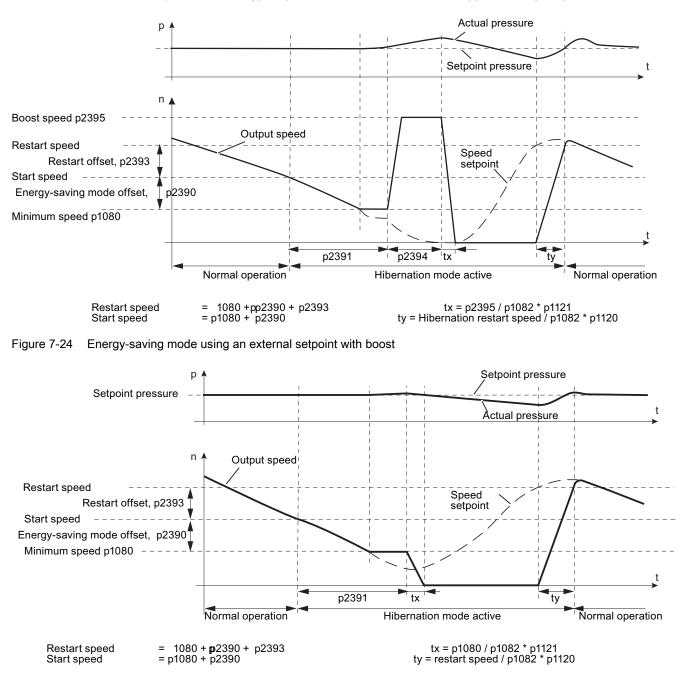
In this operating mode, the setpoint is specified by an external source (e.g. a temperature sensor); the technology setpoint can be used here as a supplementary setpoint.
