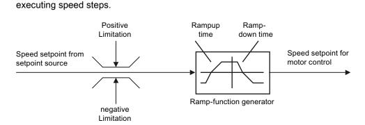
Figure 7-10 Setpoint processing in the inverter
