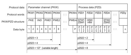
Figure 6-6 USS user data structure
