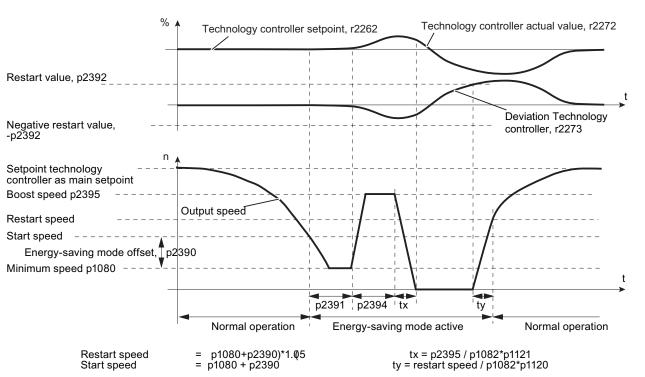
In this operating mode, the technology controller must be activated as the setpoint source (p2200) and used as the main setpoint (p2251). The function can be operated both with and without boost.
