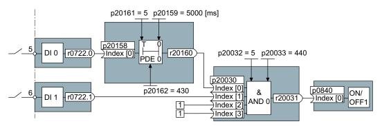
Figure 1-4 Example: Signal interconnection for interlock
