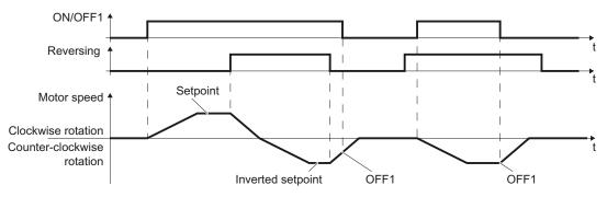
Figure 7-2 Two-wire control, method 1
