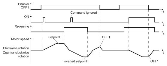
Figure 7-6 Three-wire control, method 2
