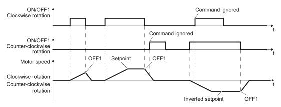
Figure 7-3 Two-wire control, method 2
