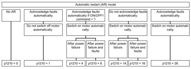
Figure 7-16 Selecting the automatic restart mode
