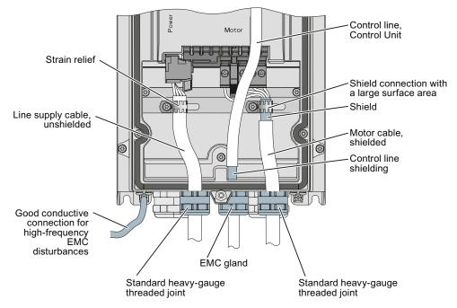
The EMC-compliant installation of the PM230 Power Module and Control Unit is shown in the following diagram.
