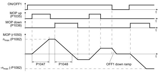
Figure 7-9 Function chart of motorized potentiometer
