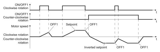
Figure 7-4 Two-wire control, method 3
