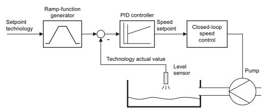
Figure 7-18 Example: technology controller as a level controller
