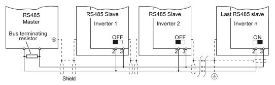
Figure 6-4 Communication network via RS485
