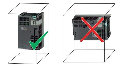
Installing Power Modules with degree of protection IP20
