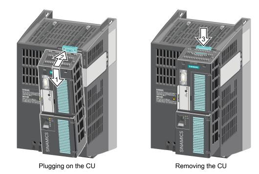
Installing the Control Unit on an IP20 Power Module
