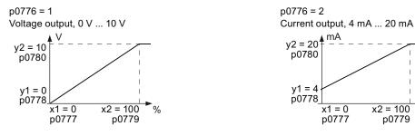
Figure 5-3 Examples for scaling characteristics
