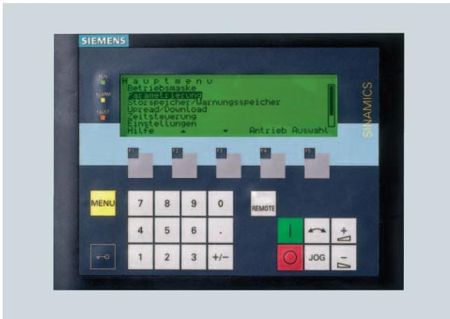
The AOP30 Advanced Operator Panel is an optional input/output device for SINAMICS DC MASTER converters. It can be separately ordered. The operator panel is only designed for installation outside the converter (e.g. in a cabinet door up to 4 mm thick), installation cut-out 141.5 × 197.5 mm.
