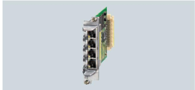
The CBE20 Communication Board can be used to connect to a PROFINET IO network via the Advanced CUD.
