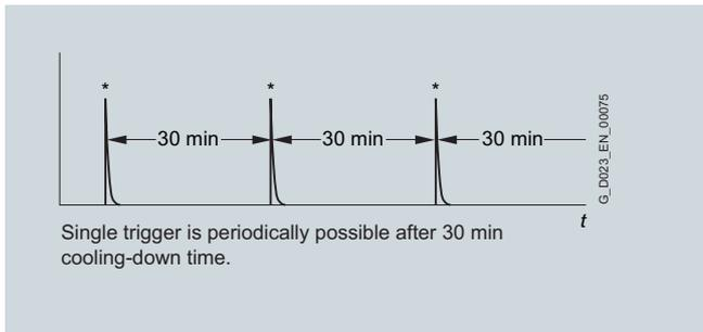
Single trigger is periodically possible after 30 min cooling-down time.
