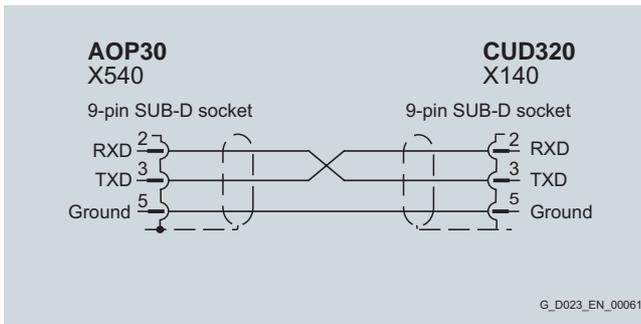
Assignment of the RS232 cable for connecting to an AC SINAMICS unit (not for SINAMICS DC MASTER!)
