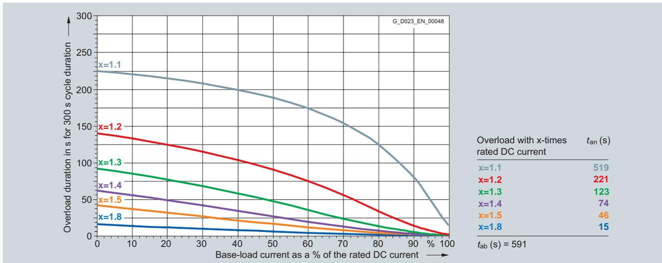
6RA8093-4DS22-0AA0 1 600 A/two-quadrant operation 400 V, 6RA8093-4DV62-0AA0 1 600 A/four-quadrant operation 400 V, 6RA8093-4GS22-0AA0 1 600 A/two-quadrant operation 575 V, 6RA8093-4GV62-0AA0 1 600 A/four-quadrant operation 575 V
