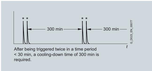
After being triggered twice in a time period < 30 min, a cooling-down time of 300 min is required.
