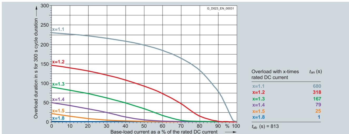
6RA8075-6DS22-0AA0 210 A/two-quadrant operation 400 V, 6RA8075-6DV62-0AA0 210 A/four-quadrant operation 400 V, 6RA8075-6FS22-0AA0 210 A/two-quadrant operation 480 V, 6RA8075-6FV62-0AA0 210 A/four-quadrant operation 480 V, 6RA8075-6GS22-0AA0 210 A/two-quadrant operation 575 V, 6RA8075-6GV62-0AA0 210 A/four-quadrant operation 575 V
