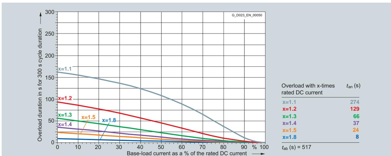
6RA8095-4DS22-0AA0 2 000 A/two-quadrant operation 400 V, 6RA8095-4DV62-0AA0 2 000 A/four-quadrant operation 400 V
