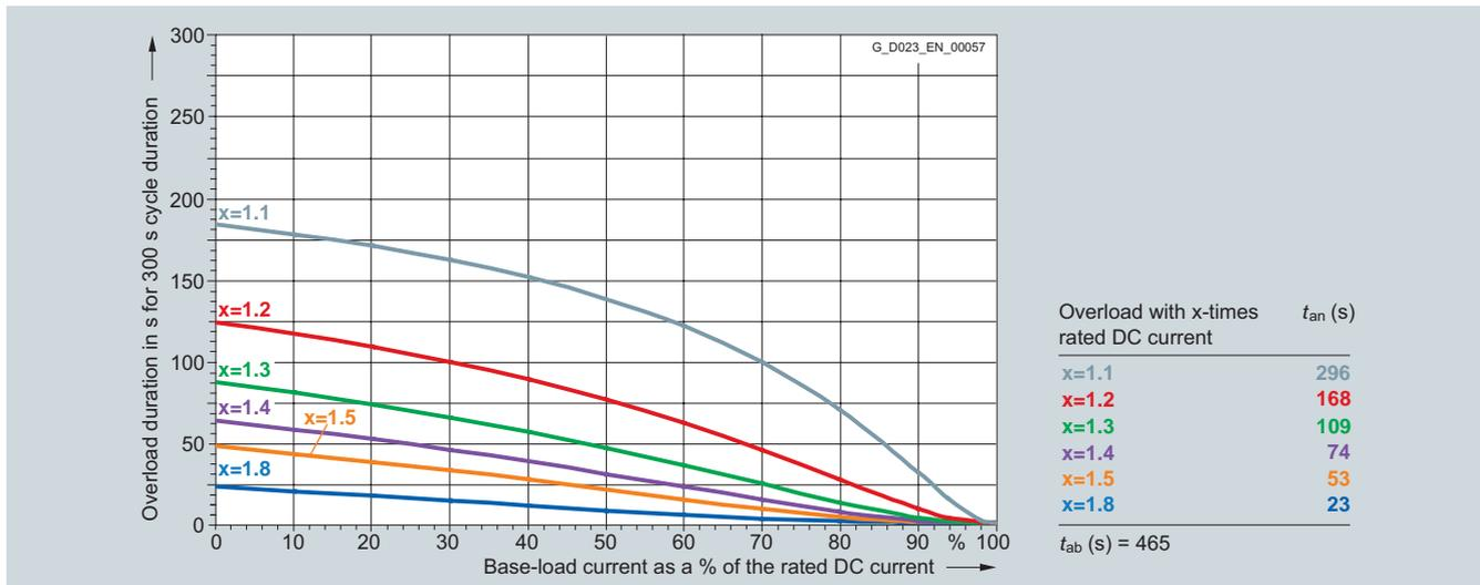
6RA8097-4KS22-0AA0 2 600 A/two-quadrant operation 690 V, 6RA8097-4KV62-0AA0 2 600 A/four-quadrant operation 690 V
