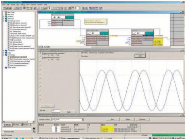
Drive Control Chart (DCC) extends the possibility of very simply configuring technological functions – both for the SIMOTION motion control system as well as for the SINAMICS DC MASTER drive system. For users, this opens up a new dimension regarding the adaptability of the systems mentioned to the specific functions of their machines. DCC has no restrictions with regard to the number of usable functions; this is only limited by the performance capability of the target platform.
