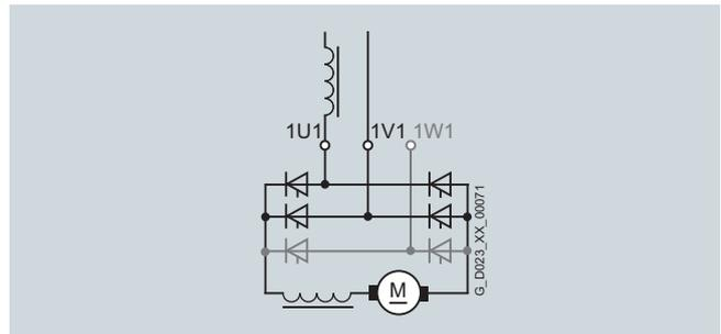
For units up to 125 A and up to 575 V AC, the full functionality is available even when supplied through just two conductors. This means, for example, that when retrofitting a converter with single-phase connection, it is not necessary to make any changes to the existing machine or plant – and the retrofitted drive system can be integrated into state-of-the-art communication concepts (TIA).
