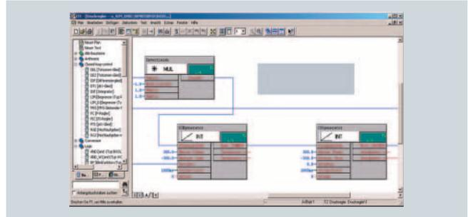
A sufficient number of free function blocks for various applications is included as standard. Optionally, the functional scope can be subsequently extended using free function blocks from Drive Control Chart (DCC). This allows the drive to be optimally adapted to the particular application – both technically and economically.
