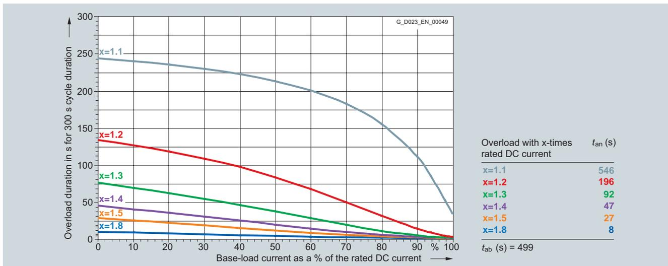
6RA8093-4KS22-0AA0 1 500 A/two-quadrant operation 690 V, 6RA8093-4KV62-0AA0 1 500 A/four-quadrant operation 690 V, 6RA8093-4LS22-0AA0 1 500 A/two-quadrant operation 830 V, 6RA8093-4LV62-0AA0 1 500 A/four-quadrant operation 830 V
