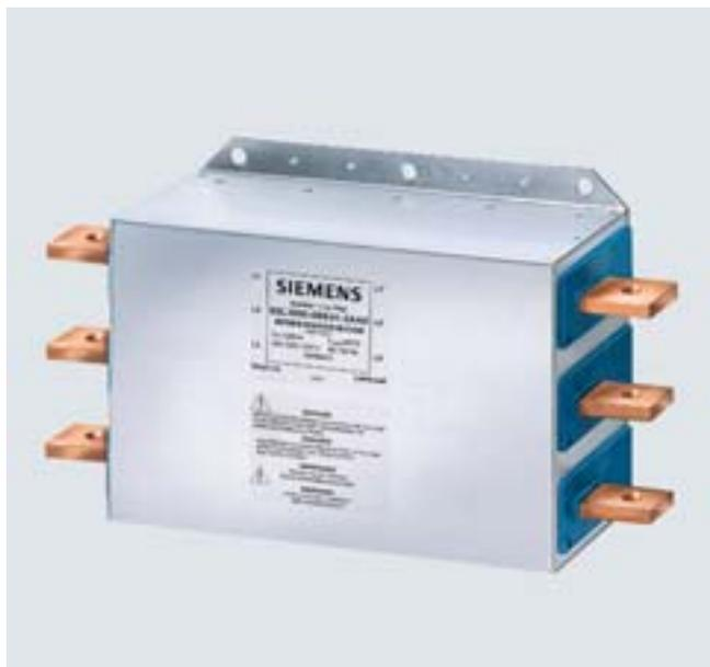
To limit the emitted interference, the drive converters are equipped as standard with a radio interference suppression filter that conforms to the limits defined in Category C3. SINAMICS G130 converters equipped with the line filter also meet the limits for use in the first environment (Category C2) as specified in EN 61800-3.<sup>1)</sup>
