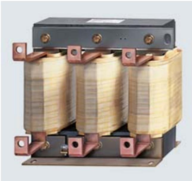
It is recommended that a line reactor is always connected on the line side of the converter, as in practice, it is often not known on which supply configuration individual converters are to be operated, i.e. which supply short-circuit power is present at the converter connection point.
