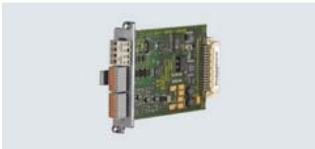
The TB30 Terminal Board supports the addition of digital inputs/digital outputs and analog inputs/analog outputs to the CU320-2 Control Unit.
