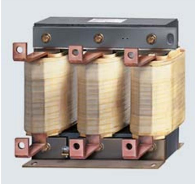
Motor reactors reduce the voltage load on the motor windings by reducing the voltage gradients on the motor terminals generated when the converter is used. At the same time, the capacitive charge/discharge currents that place an additional load on the converter output when long motor cables are used are reduced. The maximum permissible output frequency when a motor reactor is used is 150 Hz.
