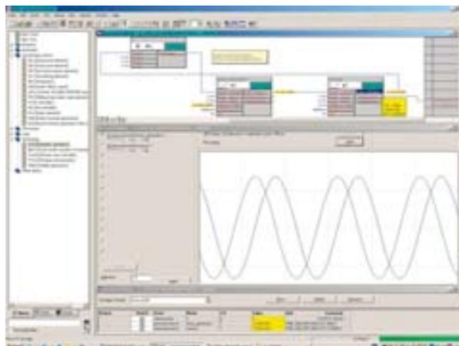
Drive Control Chart expands the facility for the simplest possible configuring of technological functions both for the SIMOTION motion control system as well as for the SINAMICS S120/S150/G130/G150 drive systems. For users, this opens up a new dimension regarding the adaptability of the systems mentioned to the specific functions of their machines. DCC has no restrictions with regard to the number of usable functions; this is only limited by the performance capability of the target platform.
