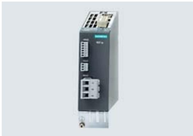
The VSM10 Voltage Sensing Module reads the voltage waveshape at the motor end. This allows the SINAMICS G130 converter to be connected to a permanent-magnet, synchronous motor without encoder ("flying restart" function).
