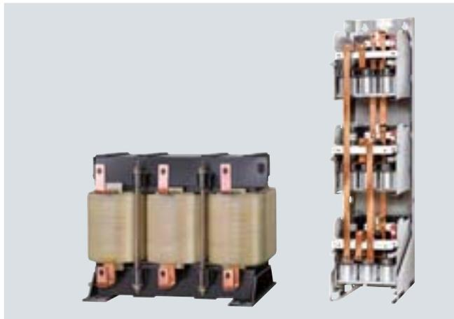
dv/dt filter plus VPL (**V**oltage **P**eak **L**imiter) limit the voltage rate-of-rise  $dv/dt$  to values  $< 500 \text{ V}/\mu\text{s}$  and the typical voltage peaks to the following values according to the limit value curve to IEC/TS 60034-17: 2006:
