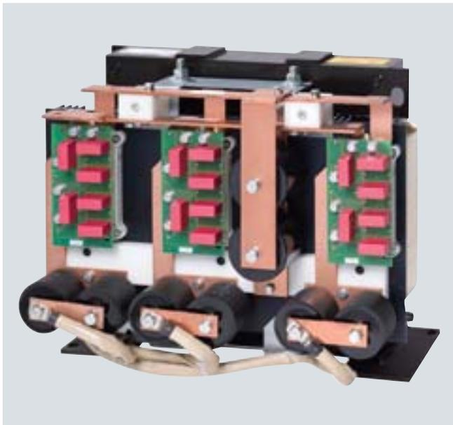
dv/dt filter compact plus VPL (**V**oltage **P**eak **L**imiter) limit the voltage rate-of-rise  $dv/dt$  to values  $< 1600 \text{ V}/\mu\text{s}$  and the typical voltage peaks to the following values according to the limit value curve A to IEC 60034-25: 2007:
